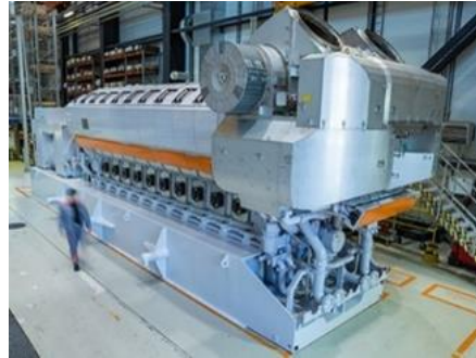
Wärtsilä 31V10DF marine engine (Full load: 5500 kW)
